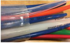
Rotary Atomizer Control Bundle with Unique Hose and Tube Markings
